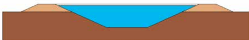
FIGUR 19: PRINCIPSKITSE FOR DAMVARMELAGER
